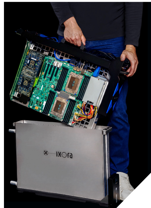
Photograph of an Ixora immersion cooling system. Source: Ixora
